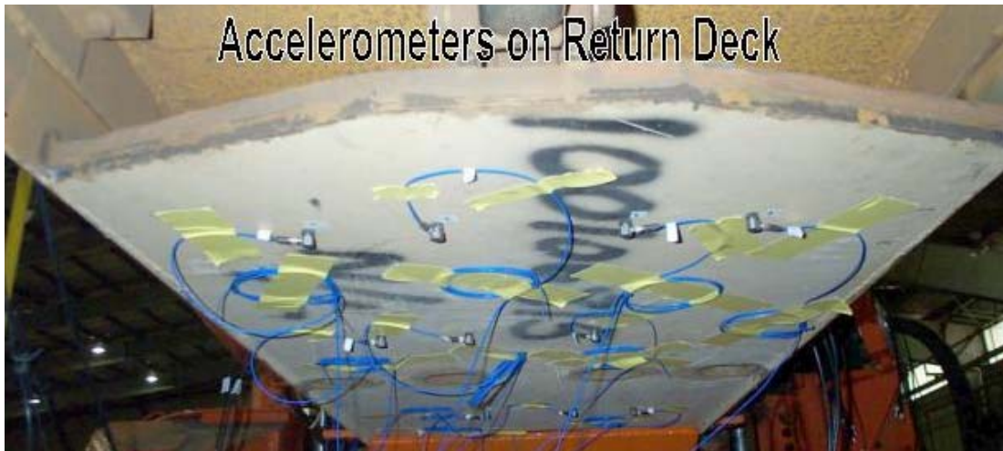
Figure 3. Accelerometer locations on the return deck of the continuous miner.
