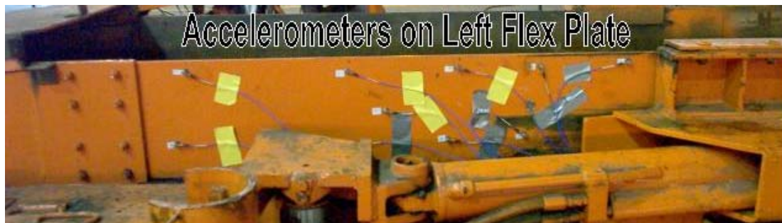
Figure 4. Accelerometer locations on the left flex plate of the continuous miner.
