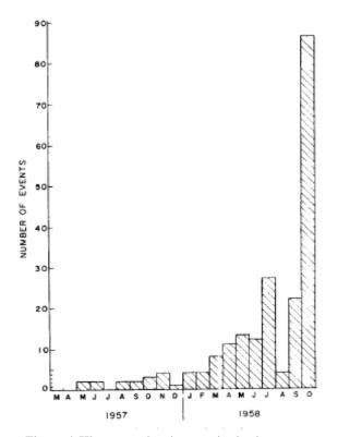
Figure 6. Histogram showing quasi-seismic events per month during mining of the last three longwalls at Springhill Mine (3).
