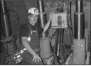
A researcher checks a continuous recording methanometer installed on longwall shields at critical locations on the active face during long-term emission studies.
