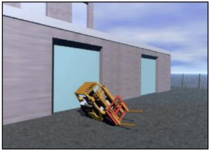
Poor lift-truck operating practices, such as high-speed turns, can lead to serious accidents.
