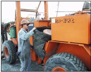
A mechanic removes sound absorption material from a motor to prepare for a noise measurement with an uncontrolled source.
