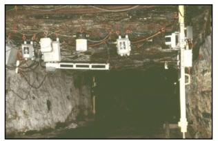
Mine fire sensor array in the Safety Research Coal Mine.
