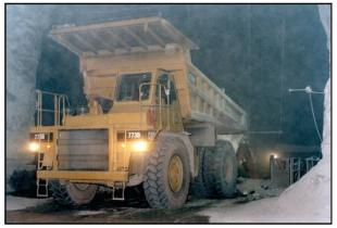
Haul truck dumping at a crusher in an underground limetone mine.
