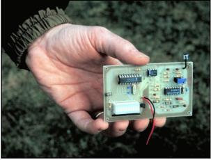
Prototype of inexpensive personal noise dosimeter.
