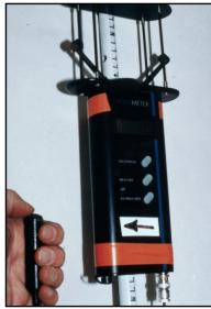
Handheld ultrasonic anemometer capable of measuring very low air velocities.
