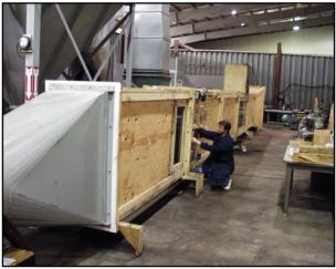
Wind tunnel used to evaluate shield dust entrainment.
