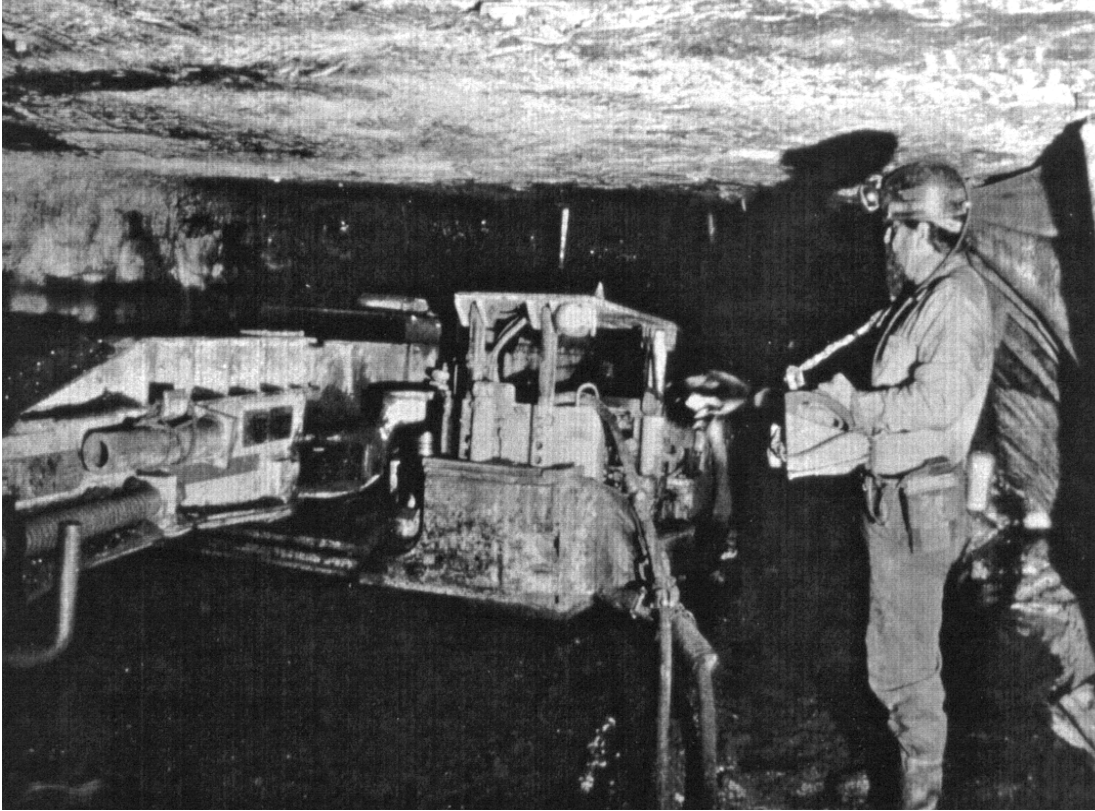
Figure 2. - Miner operating a continuous mining machine by remote control
