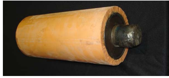
(b) Urethane coated tail roller.
