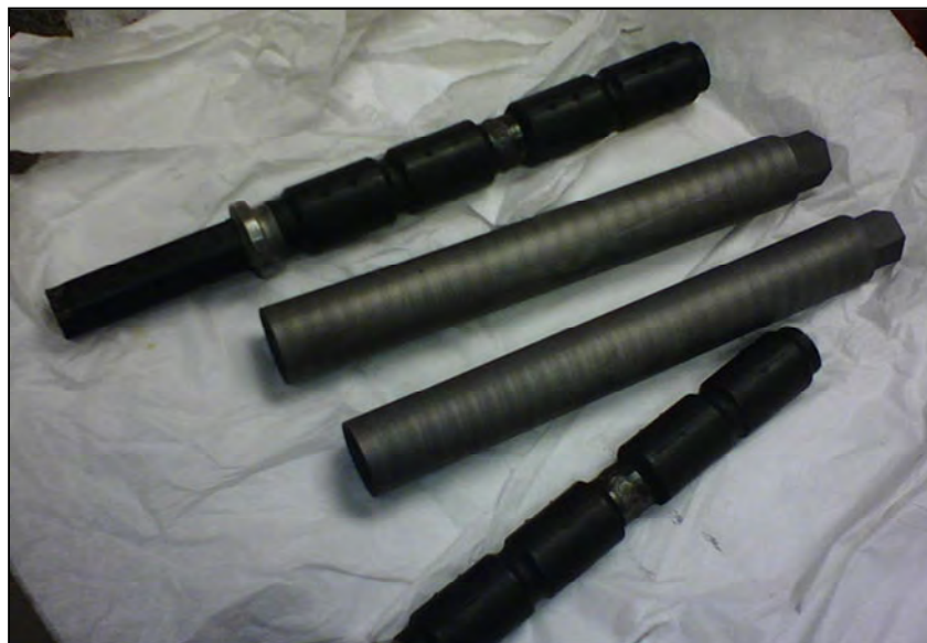
Fig. 4 – Picture of bit isolator design, two units disassembled.
