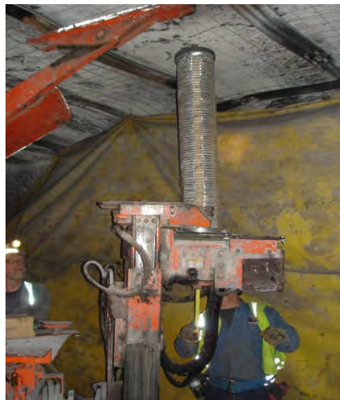
Fig. 9 – The CDSE installed on a roof bolting machine. At this point in the drilling process, the drill chuck has been raised far enough that the top of the CDSE has come into contact with the mine roof.
