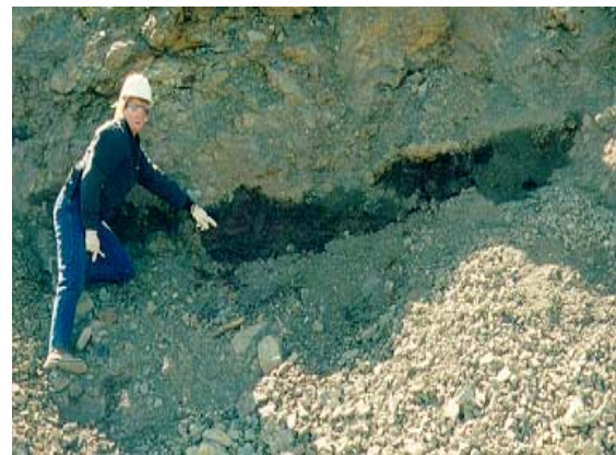
Figure 8. Seep in failing slope.
