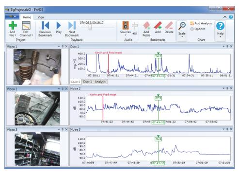
This screenshot from the EVADE 2.0 software shows the expanded multi-channel capabilities of the program. In this example, three separate video channels have been created and are displayed next to their associated exposure plots.
