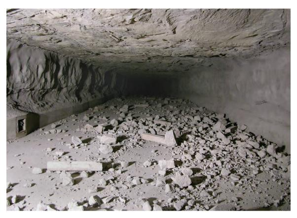
Figure 73.—Debris after Test 6 (LLEM #506) looking outby from ~1,050 ft.
