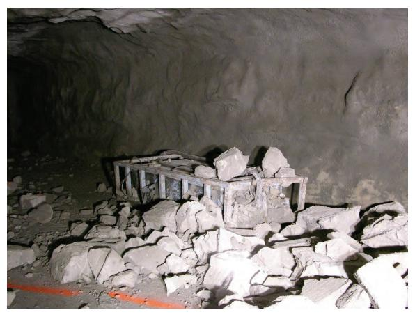
Figure 53.—Final location of battery charger near 720 ft after Test 5 (LLEM #505).
