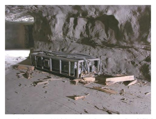
Figure 12.—Battery charger and debris from the wood cribs near X-7 after Test 1 (LLEM #501).
