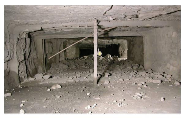
Figure 42.—Debris from X-3 seal after Test 5 (LLEM #505) looking into X-3 toward B-drift.
