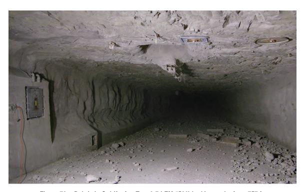
Figure 70.—Debris in C-drift after Test 6 (LLEM #506) looking outby from 757 ft.
