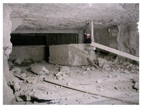
Figure 18.—Remains of X-3 seal viewed from C-drift after Test 2 (LLEM #502).
