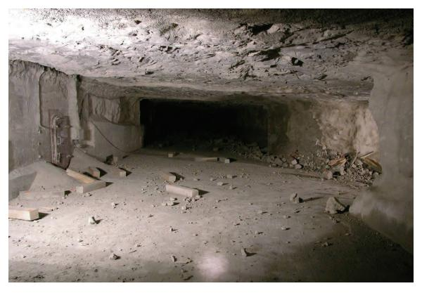
Figure 46.—Debris in C-drift after Test 5 (LLEM #505) looking outby toward X-4 (right side of photo) at 355 ft.
