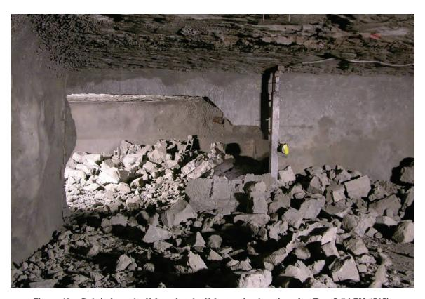
Figure 43.—Debris from the X-3 seal at the X-3 stopping location after Test 5 (LLEM #505).
