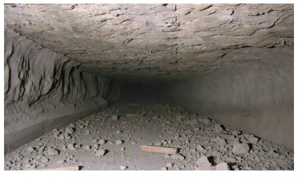
Figure 71.—Debris in C-drift after Test 6 (LLEM #506) looking outby from ~850 ft.
