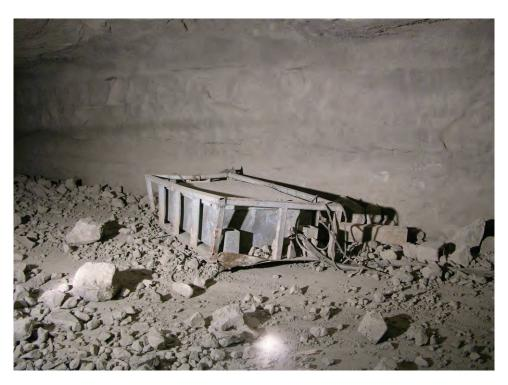
Figure 77.—Final position of battery charger after Test 6 (LLEM #506).
