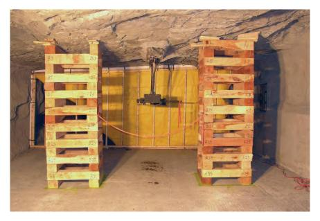
Figure 10.—Wood cribs at 312 ft looking inby in C-drift before Test 1 (LLEM #501).
