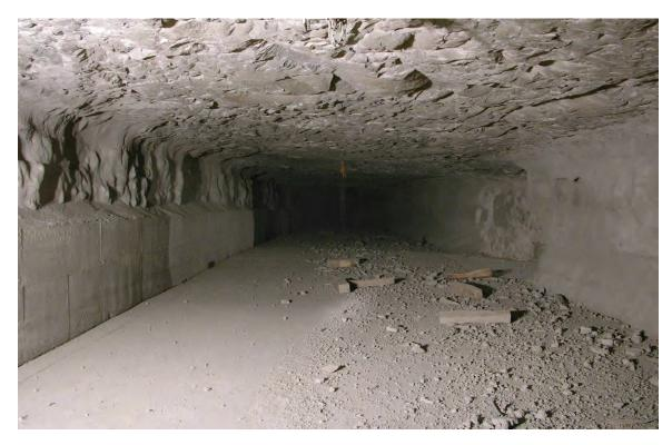
Figure 68.—Debris in C-drift after Test 6 (LLEM #506) looking outby from ~500 ft.
