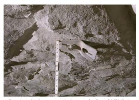
Figure 82.—Belt hanger at 403 ft after explosion Test 6 (LLEM #506).
