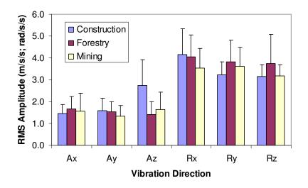
Figure 1.—Multiaxis vibration exposures during routine machine operation (rms amplitude, average, and standard deviation).
