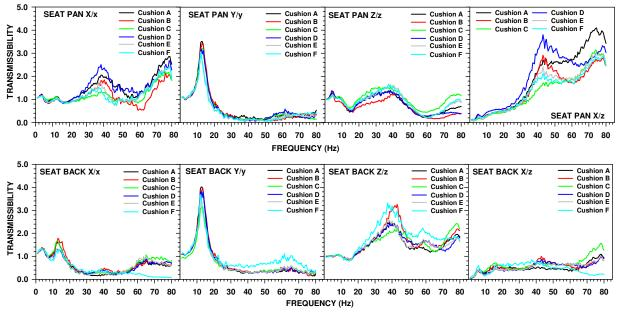
Figure 1.—Mean seat pan and seat back transmissibilities (seven subjects).
