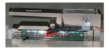
Figure 1.—The MRI-compatible flextensional piezoelectric actuator is constructed of titanium and sheets of piezoelectric material (black arrow) that bend in response to applied voltage to cause vertical translation of the lever arm platform.
