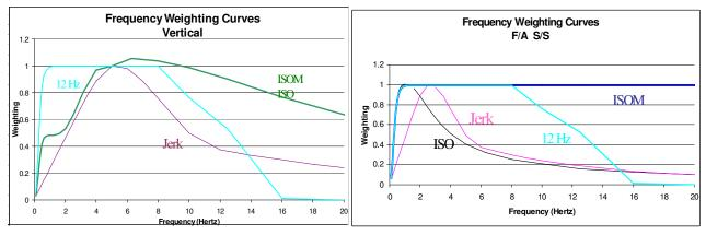
Figure 1.—Frequency weighting curves. (F/A = fore/aft; S/S = side/side.)
