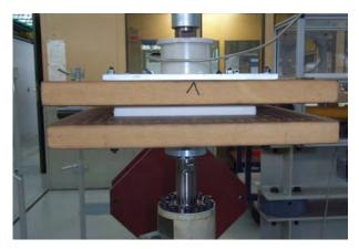
Figure 1.—Hydraulic test rig with foam.
