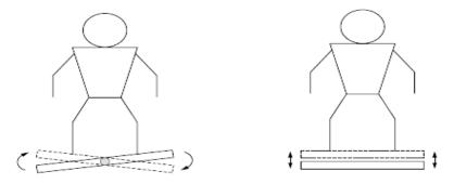
Figure 1.—Oscillating versus vertical vibrating plates.
