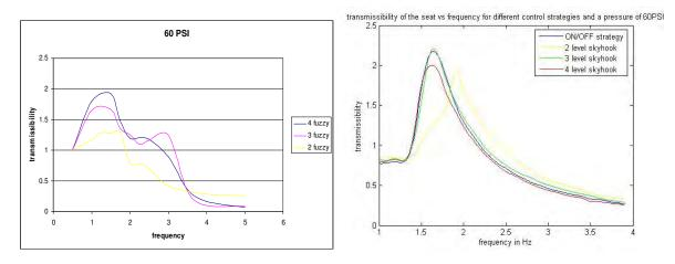
Figure 2.—Transmissibility of the seat with a fuzzy controller (left) and a discrete controller (right).
