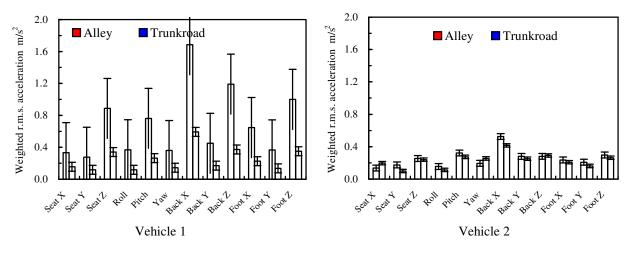
Figure 3.—Frequency-weighted rms acceleration for each axis.
