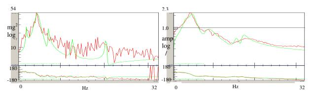
Figure 1.—Vertical cushion output (red) amplitude (*above*) and phase (*below*) fitted with five modes of an operational modal analysis (green).
