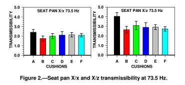
BPF. The seat base transmissibility results did indicate that the E-2C seat structure was not rigid, particularly in the Y axis, and most likely influenced the behavior at the seat/occupant interfaces. The transmissibility data can be used to predict the multiaxis accelerations entering the human during operational exposures and target seat vibration mitigation strategies.
