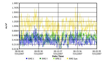
Figure 2.—Results of one 20-min period during residential solid waste collection.
