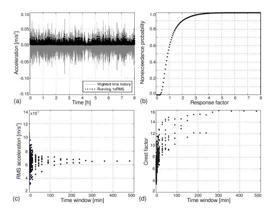
Figure 1.—(a) 8-hr weighted time history; (b) cumulative probability of response factor; (c) rms acceleration; (d) crest factor as a function of time window.
