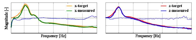
Figure 3.—Amplification functions  $V_m(s)$  for x and z, target and measurement.
