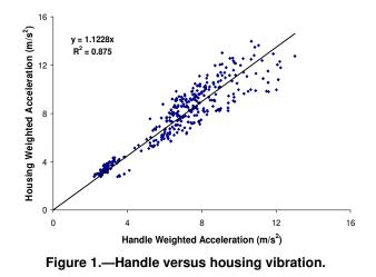
Both the current and proposed impact wrench assessment standards call for testing by three tool operators. However, a power analysis [Montgomery 2001] revealed that three tool operators may not be enough for reliable tool screening. Based on the acceleration variance observed in this study, at least five tool operators would be required to reliably rank-order all five tool models using this revised procedure ( $\alpha = 0.05$ ,  $\beta = 0.20$ , p < 0.05).
