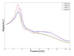
Figure 5.—Seat transfer functions  $H_S(s)$  for different foams.
