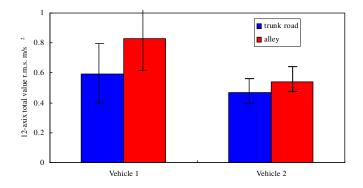
Figure 2.—Total vibration values obtained for two types of day care vehicles.
