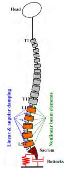
Figure 1.—Finite-element model.
