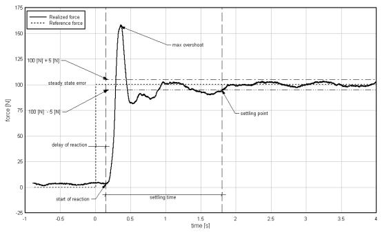
Figure 1.—Exemplary time history of step reference and forces realized by human operator.
