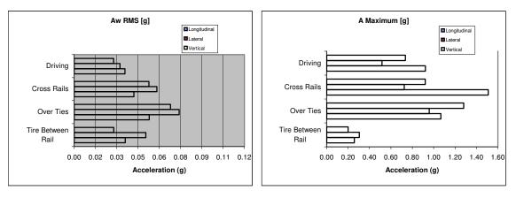
Figure 1.—Weighted rms acceleration.
