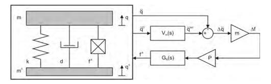
Figure 2.—Equivalent model of the active ground-excited SDOF.
