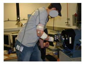
Figure 2.—Measurement of the transmissibility on a 1-D test system.
