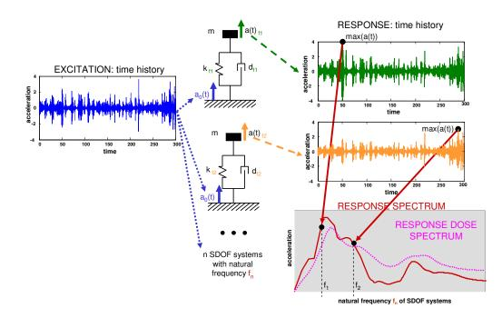
Figure 1.—Calculation of the response spectrum and the response dose spectrum [Gupta 1990].
