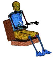
Figure 2.—Simplified seat with CASIMIR.
