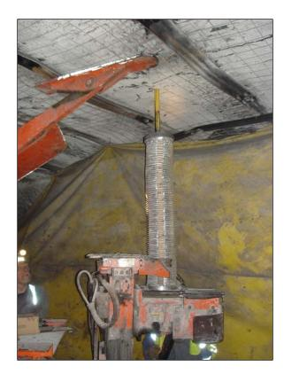
Figure 1.—The CDSE at the start of drilling. The gap above the CDSE allows the operator to see the drill bit/media interface to start the hole. The height of the CDSE can be varied to suit the particular application.
