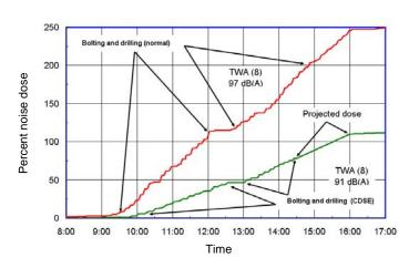
Figure 5.—Field data show that using a CDSE reduced a roof bolting machine operator's 8-hour time-weighted exposure from 97 to 91 dB(A).
