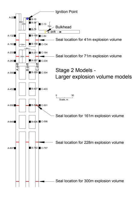
Figure 17.—Layout of large-volume confined explosion models.
