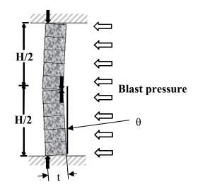
Figure 27.—One-way arching failure mechanism in Wall Analysis Code (WAC).
