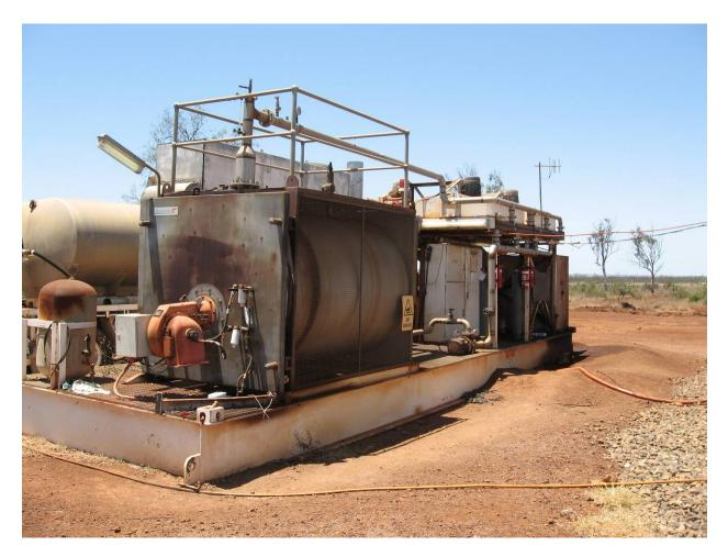
Figure 9.—Tomlinson boiler for inertization at an Australian coal mine.
