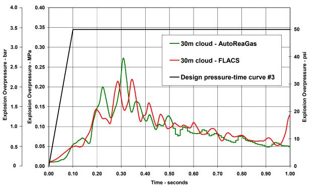
NIOSH Design Pressure-Time Curve #3 - Limited Volume, Unconfined Pressures are Overpressure
