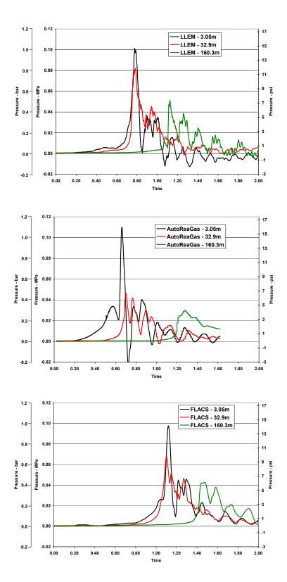
Figure 16.—Calibration experiments and calculations compared. *Top:* Lake Lynn Experimental Mine calibration data; *center:* calculations from AutoReaGas model; *bottom,* calculations from FLACS model.
