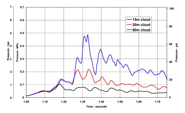
Figure 21.—Calculated pressure-time histories at seal for "leaking seal" explosion models using AutoReaGas (*top*) and FLACS (*bottom*).
