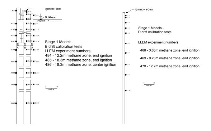
Figure 15.—Layout of calibration models in the LLEM. *Left:* B-drift calibration tests; *right:* D-drift calibration tests.
