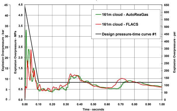
NIOSH Design Pressure-Time Curve #1 - Unlimited, Confined Volume Pressures are Overpressure
