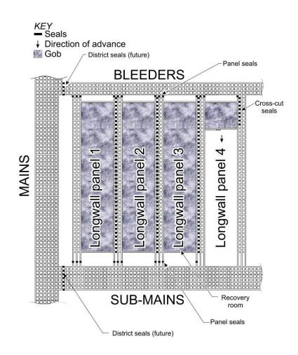
Figure 5.—Typical layout of longwall mining with immediate panel sealing. Also shown are typical locations for district, panel, and crosscut seals.
