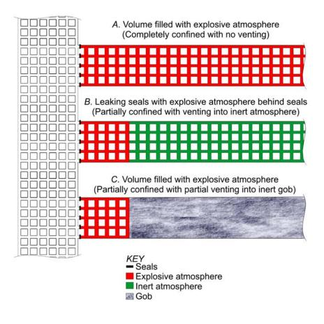
Figure 7.—Three general types of explosive gas accumulation within sealed areas.
