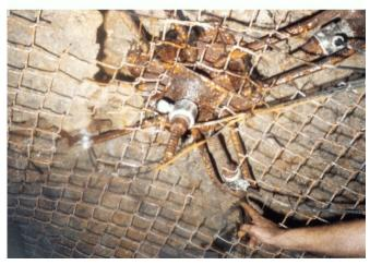
Figure 17.—Load cells at truss four-way bracket.
