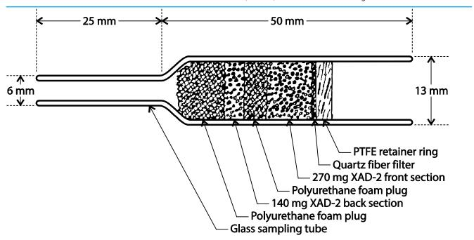
Figure 2. OVS-2 Sampler
