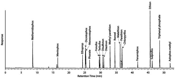
Figure 3. Typical chromatogram of organophosphorus compounds
