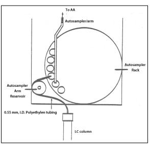
Figure 1 HPLC/AAS interface system
