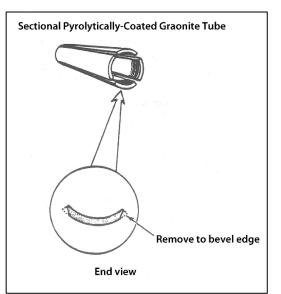
Figure 2 Construction of a laboratory made platform
