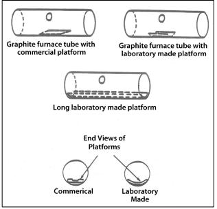
Figure 3 Placement of commercial and "laboratorymade" graphite L'vov platforms in furnace tubes.
