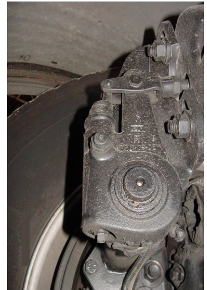
Photo, right. Automatic Slack Adjuster as a component of the foundation brakes.
