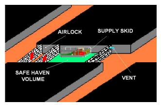
safe haven or zone. The breathable air systems needed for the safe havens are supplied by either compressed air cylinders located on the supply skid, vertical boreholes drilled from the surface into each safe haven area, or compressed air lines, which are protected against explosive forces, and typically are located along the track or belt line.
