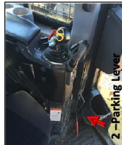
Parking lever (2). (Photo courtesy of WV OSHA)
