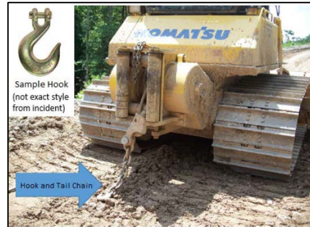
Tow hook and tail chain, showing length of towline at time of incident. (Photo courtesy of WV OSHA.)
