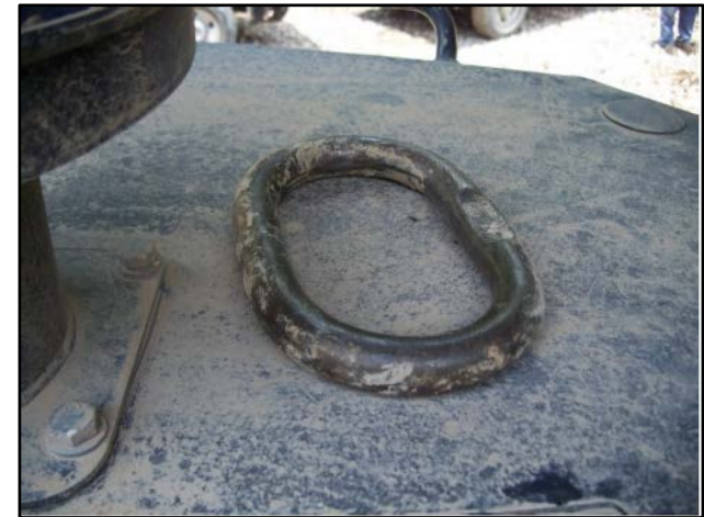
D-ring needed for connection between hook and hitch pin. (Photo courtesy of WV OSHA.)
