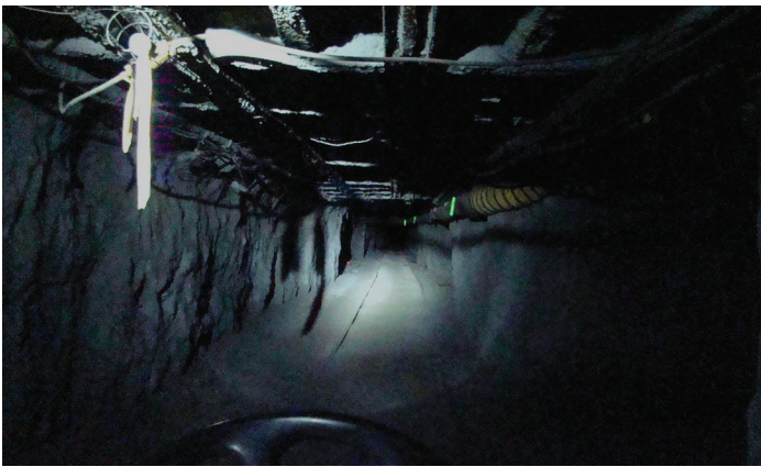
Figure 1: (Left) Illumination provided by an LED cap lamp in an underground mine. (Right) The improved illumination provided by the NIOSH-developed LED cap lamp.
