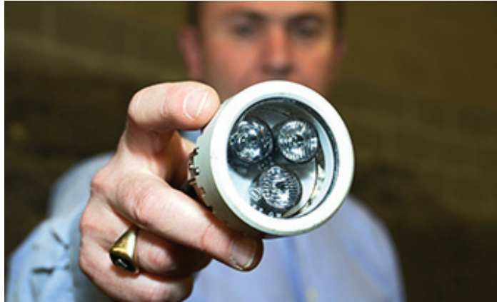
Figure 2: The NIOSH LED cap lamp uses multiple LEDs as the primary light source for better illumination distribution.
