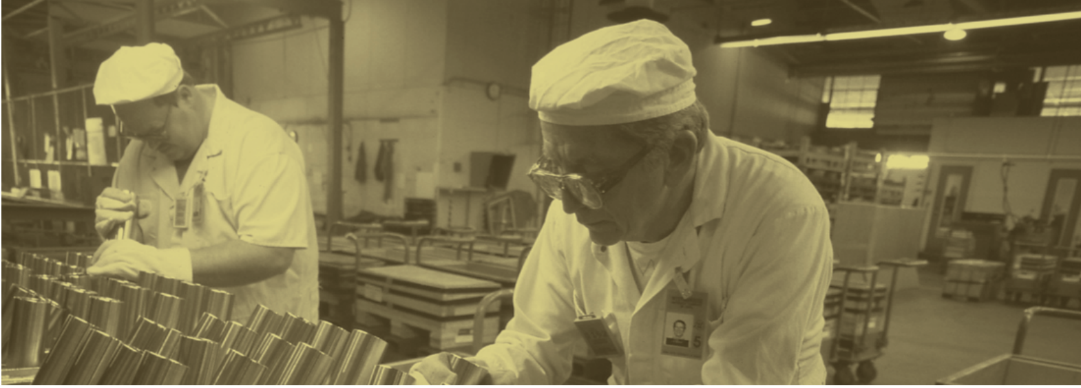
Department of Energy workers inspect uranium metal reactor fuels as part of the final product inspection process. Plant 6, Fernald Feed Materials Production Center. Photo from the U.S. Department of Energy
