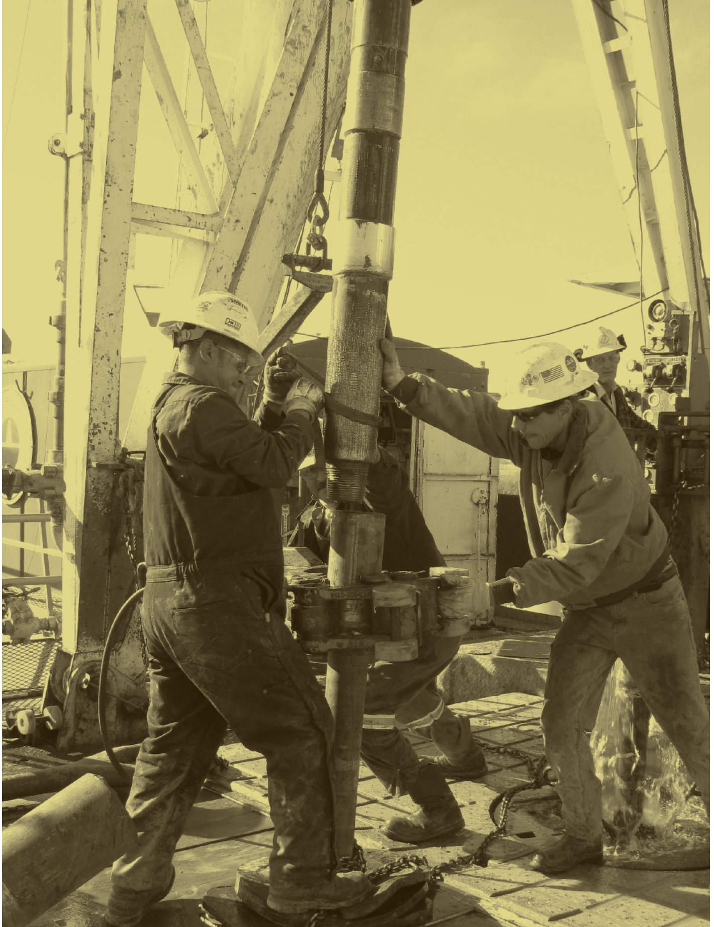
Two roughnecks work on the rig floor to drill a new oil well. These floor hands are attaching a new length of pipe to the drill.
