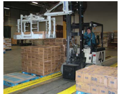
Special attachments are available for removing cartons layer by layer.
