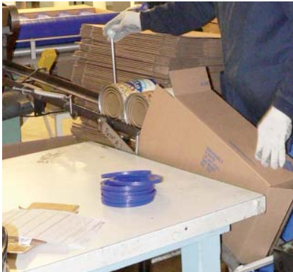
Design a conveyor system that delivers the container directly into position for loading.
