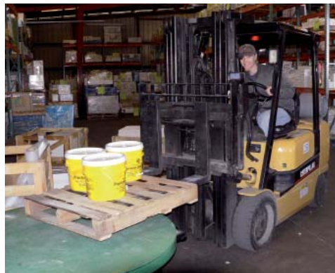
A forklift moves pallets long distances.
