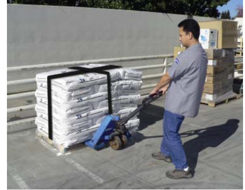
For unstable pallet loads, wrap straps around the load.
