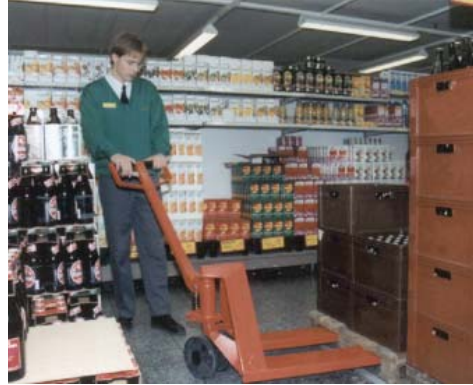
When using hand pallet trucks, be sure the floor is smooth and free of debris.
