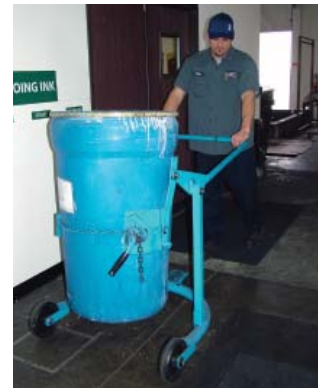
This drum dolly lifts and transports drums.
