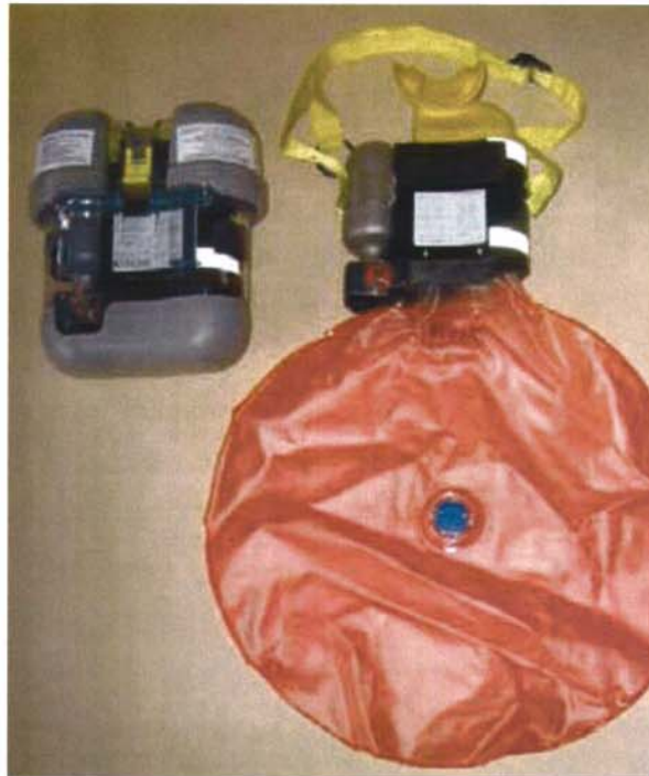
Figure 7. Partially Uncased and Uncased Ocenco M-20 Self-rescuer
