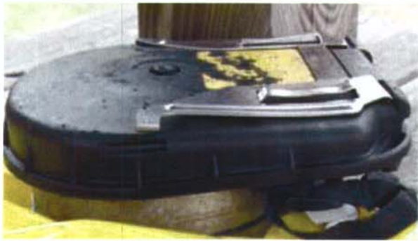
Figure 9. Dented Draeger OXY K-Plus Belt-Clip
