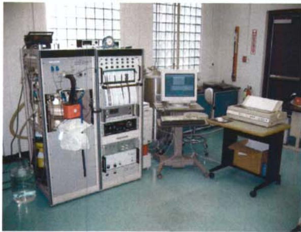
Figure 1. Breathing and Metabolic Simulator
