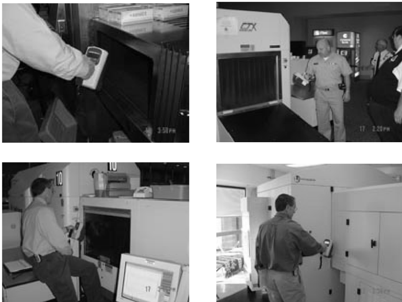
Photos 7-10: NIOSH researchers measuring radiation levels from TRX and EDS machines:
