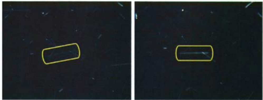
Figure 99. Field of View: 0.5mm; 11 degree extinction angle.
