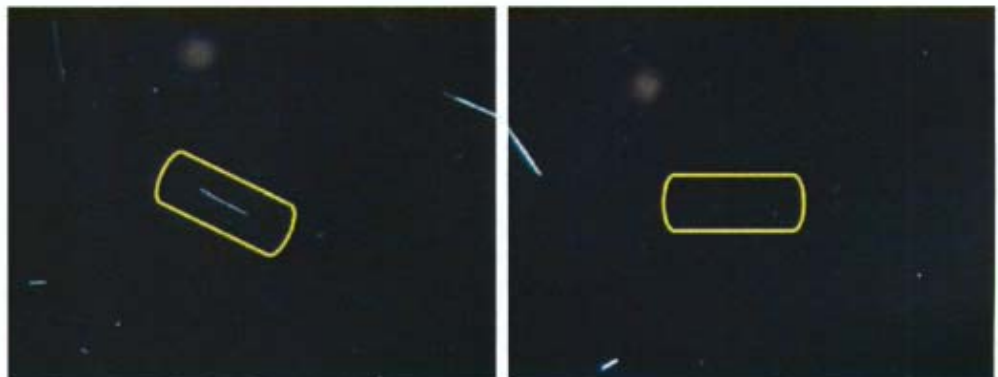
Figure 94. Field of View: 1.0mm; Parallel extinction.
