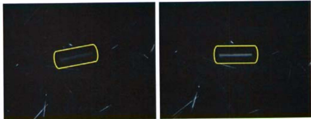
Figure 97. Field of View: 0.5mm; 11 degree extinction angle.
