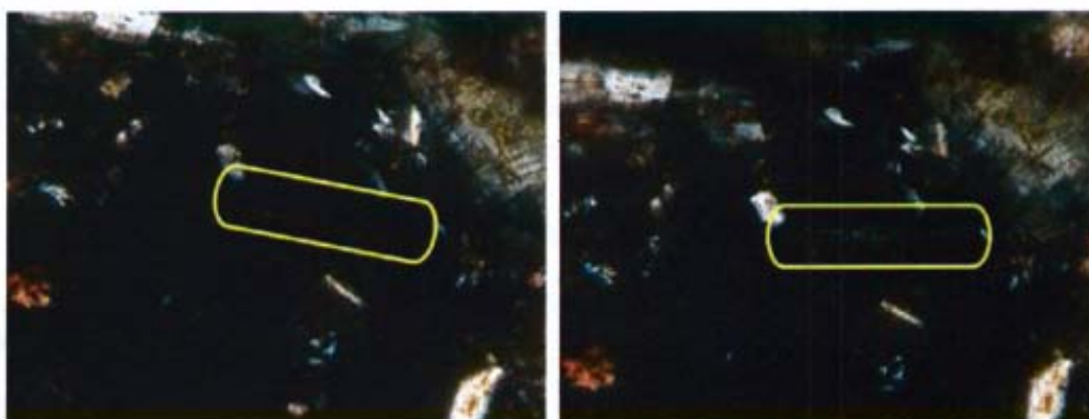
Figure 137 Field of View: 0.25mm; 12 degree extinction angle.
